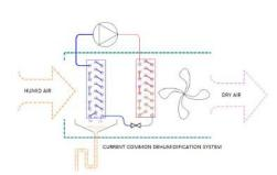
Current dehumidification process the humid air first enters the evaporator to cool down and remove moisture, then enters the condenser to be re-heated to lower the relative humidity.
