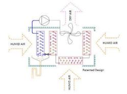
Patented 3 ways Dehumidification System, 1/3 of the humid air enters the evaporation side for dehumidification and then to be re-heated. The remaining 2/3 of the humid air helps to dissipate heat at the condenser, this increase the efficiency of the evaporator to achieve lower dew point temperature thus will remove more moisture from the humid air.
