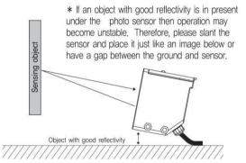
Regarding the installation direction of photo sensor, please consider about the moving direction of sensing object and install it (please refer to an image below)
