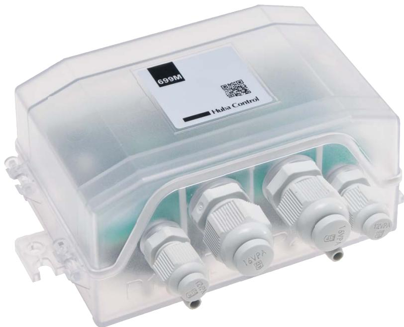
The pressure transmitter 699M is used primarily for the monitoring of air and neutral gasses. The unit is optionally available with one or two differential pressure sensors, which allows the observation of differential pressure or volumetric flow at two individual points in the system. This makes the 699M ideally suited for a multitude of tasks in the HVAC industry.
