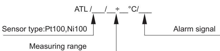
Example: temperature transmitter ATL, sensor type Pt100, measuring range 0...100°C, alarm signal 23mA.
